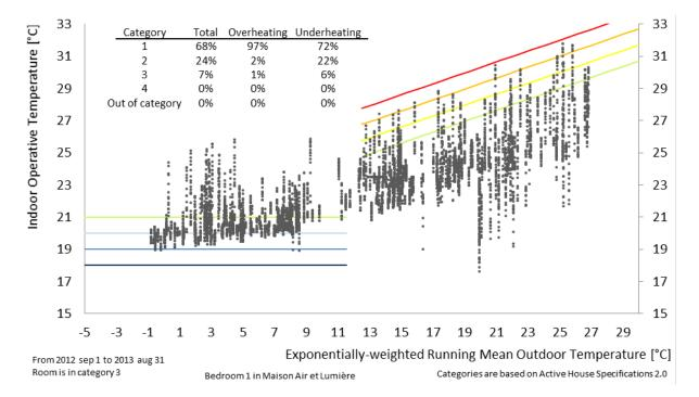
Figure 1. Measured temperatures in the master bedroom of the Maison Air et Lumiere, active house n°3, and evaluated in categories according to Active House Specification, based on the adaptive comfort method and criteria from EN 15251.
